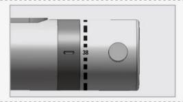
Screw the regulation knob screw and tighten it.
