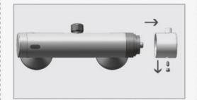
Proceed to achive a38°C settings by turning the spindle and measuring the water temperature with a thermometer.
